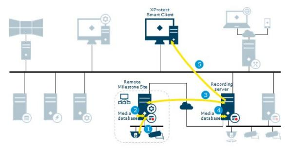
Illustrates when recording is done on both sites. Recordings can be retrieved to the central site based on schedule, event or request. XProtect Smart Client users, specified for the interconnected system, only need to log into the management server on the central site to view video.
