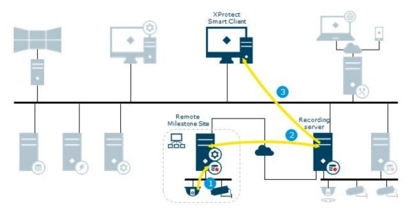
Illustrates how XProtect Smart Client users, specified for the interconnected system, only need to log into the management server on the central site to view video.
